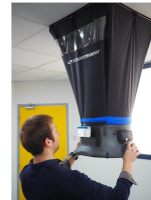
Use of the air flow meter
